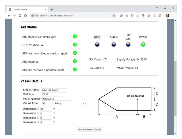
A series of simple Tick and Cross icons give an immediate indication of correct operation and you also have the RX and TX count to show how many targets have been received and how many successful transmissions the AIT5000 has made.
