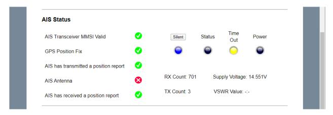
To start transmitting again, simply click the "Silent" button again and the blue "Silent" LED will go off and as soon as the AIT5000 makes its next transmission the green "Power" LED should illuminate, and this indicates that everything is working correctly, with all self-tests passed.
