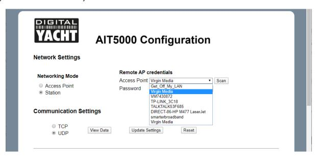
By default, the AIT5000 transmits wireless NMEA data in UDP mode which is the easiest mode to setup in most apps – just tell the app that the UDP data is on port 2000 and it should start receiving data. In some apps, such as the popular Navionics Boating app, the AIT5000 will even be detected automatically and no app setup is required.
